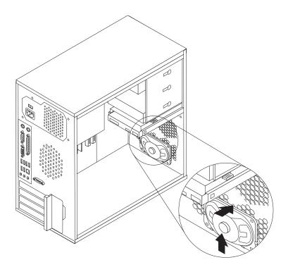
Figure 33. Removing the old internal speaker
